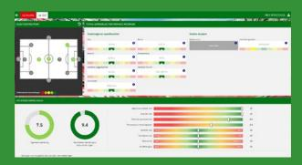
The measured data of the **HiPSter** will be automatically uploaded to the dashboard as soon as there is a stable Wifi connection. In the **Dashboard** an Al engine is running to generate the trend analyses and pitch predictions. As the **Dashboard** is an open platform also integration with other tools is possible as well as possibility for manual logging of data and reporting.
