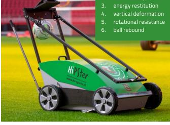
The sensors in the Hipster, a compact device the size of a family lawnmower, does all these measurements in one go. All the information obtained in this way goes automatically straight to the **Dashboard**, where results are displayed in trend figures and further analysis can take place.
